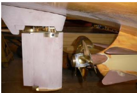
Figure 5. Model rudder-propeller arrangement.
