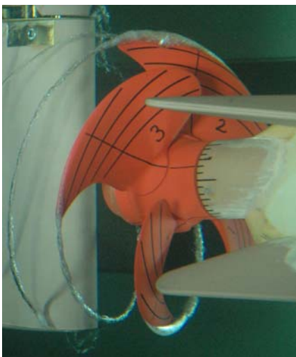
Figure 42. Vizualization of the tip cavitation on the propeller blades.
