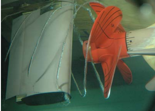
Figure 41. Visualization of tip vortices during cavitation test.
