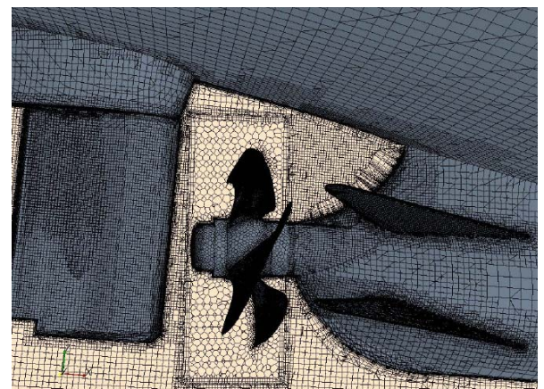
Figure 7. Computational grid on hull and propeller.
