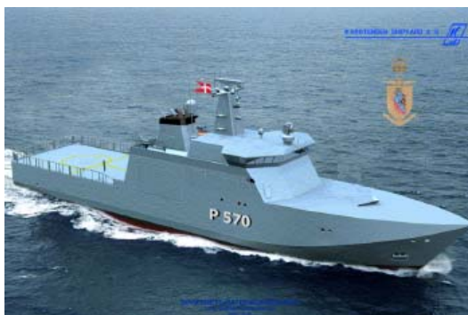
Figure 4. 70m inspection vessel.
