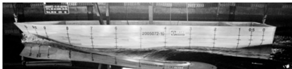
Figure 21. Wave profile on hull surface from model testing. Speed is 16kn.
