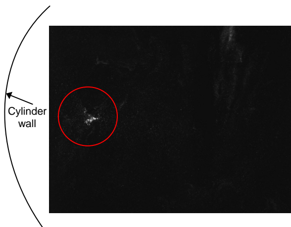
Figure 4— Wall Reflections view from backward scatter camera (Cylinder wall location is an illustration and not in true scale)
